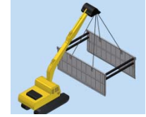
STAND TRENCH SHIELD IN UPRIGHT POSITION AND PREPARE FOR INSTALLATION
