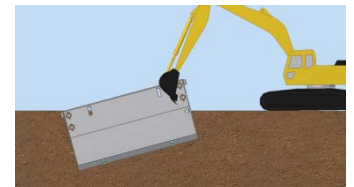
EXCAVATE SOIL WITHIN THE SHIELD AND REPEAT PREVIOUS PROCESS
